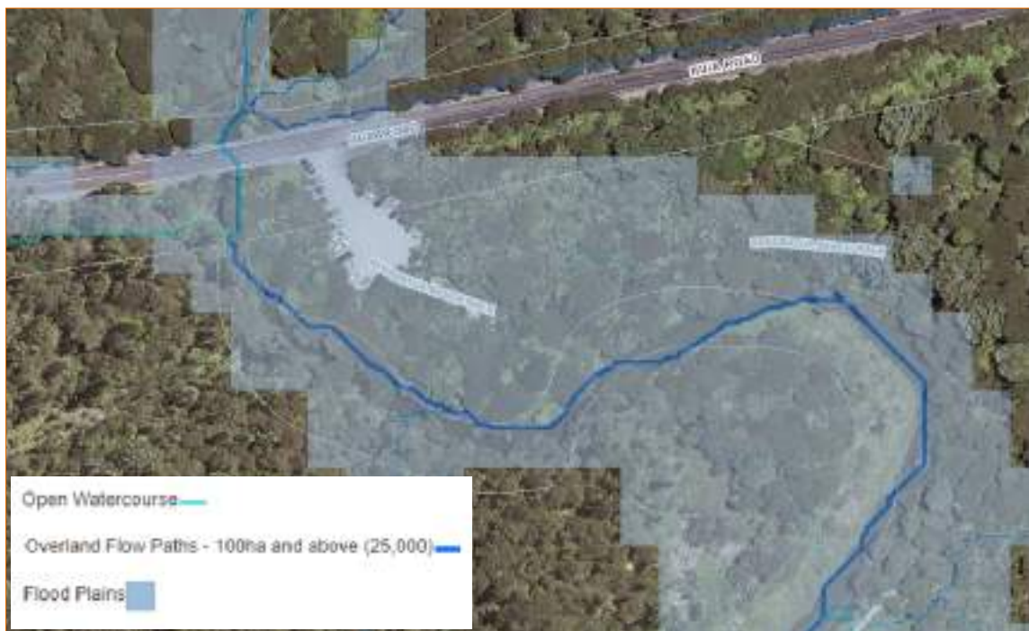
Figure 4-8: Car park located within flood plain. (Source: Auckland Council GeoMaps)
